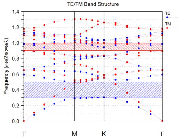
Fig. 2. Schematic of band structures.
