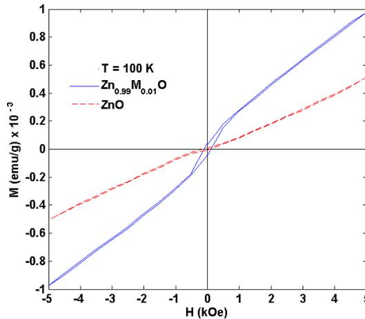
Fig. 1. Magnetization loops of ZnO and  $\text{Zn}_{0.99}\text{Mn}_{0.01}\text{O}$  at temperature 100 K
