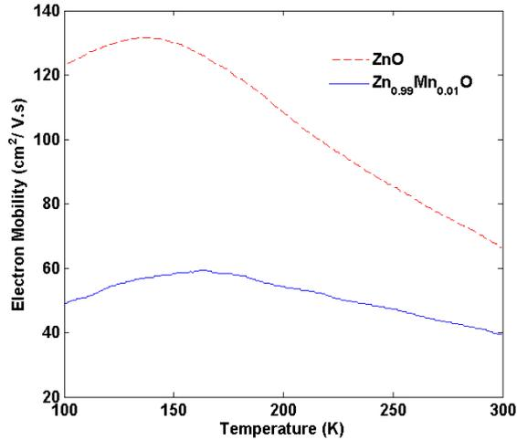
Fig.2. electron mobility for pure ZnO and Zn<sub>0.99</sub>Mn<sub>0.01</sub>O
