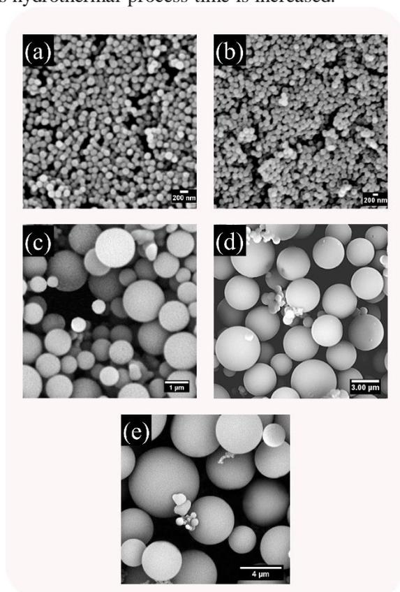
Fig. 1. SEM images of carbon nano-micro spheres
