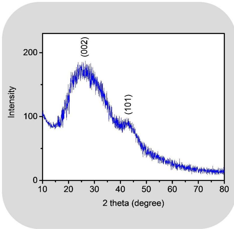
Fig. 3. XRD pattern of the obtained carbon spheres (0.75mol/lit) at 160°C for 23 h.
