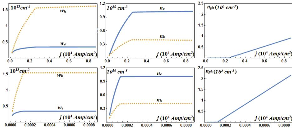
Fig. 2. Electron and hole densities in the wetting layer (left column,  $w_e$ : solid line,  $w_h$ : dashed line), electron and hole densities in the quantum dots (middle column,  $n_e$ : solid line,  $n_h$ : dashed line) and photon density in the cavity (right column) for steady-state behavior of indirect pumping (upper row from Eqs. (1)) and direct pumping (lower row from Eqs. (4)).
