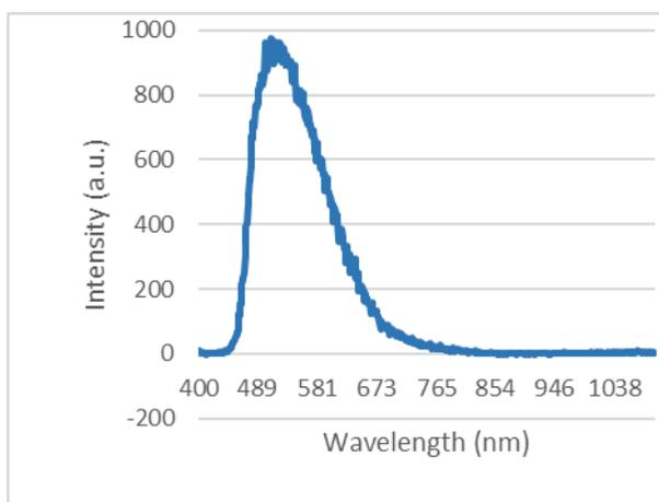
Fig. 4. Emission spectrum of the CdSe quantum dots; excitation wavelength 400 nm has been considered.
