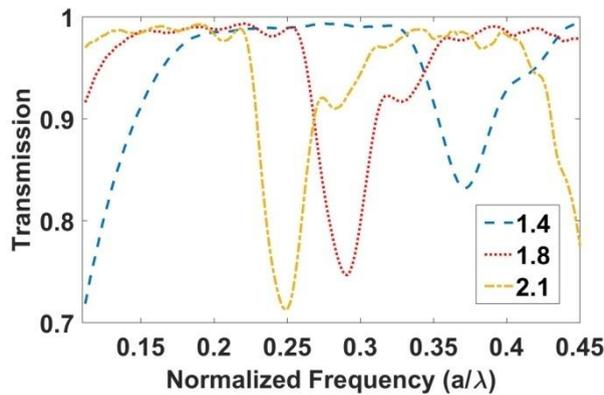
Fig. 5. The transmission spectrum of parabolic GRIN PC structures with different refractive index of background material calculated by the FDTD method
